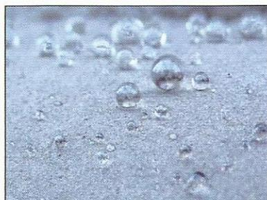
As a result of the superior characteristics of Si-COAT 570 & 570hs, the coating quickly achieves a state of Ultra-Hydrophobicity. The bio-mimicry of Si-COAT technology allows for very high contact angles between the coating and water droplets, as can be observed in nature in lotus leaves.
